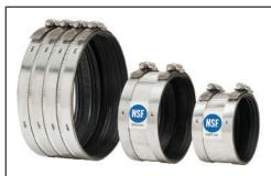
**No-Hub Couplings** Size Width No. of Torque Clamps 1.5"-4" 2.125 2 60 5" & 6" 4 60 3.0 4.0 4 8" & 10" 60 12" & 15" 5.50 6 80
